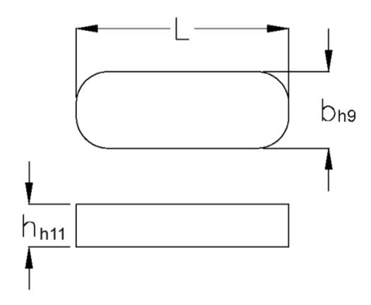
$\begin{array}{ll} b & = 10 \\ h & = 8 \\ L & = 80.0 \\ Tolerance \ b = 0.036 \\ Tolerance \ h = 0.090 \end{array}$
